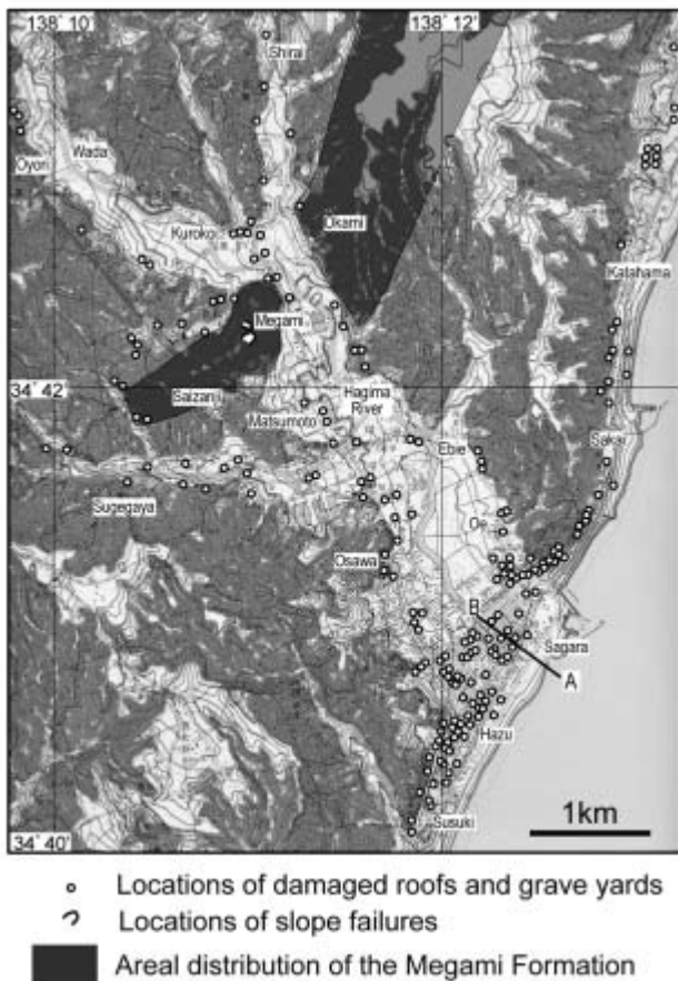
Fig. 8 Damage distribution of Sagara area in Makinohara City. The base map is used the 1/25,000 geographical map of Sagara published by Geographical Survey Institute of Japan. Contour lines are drawn by 2m under 50m high and 10m over 50m, and from the Digital Map 10m Grid (Elevation) of Sagara published by Geographical Survey Institute of Japan.
